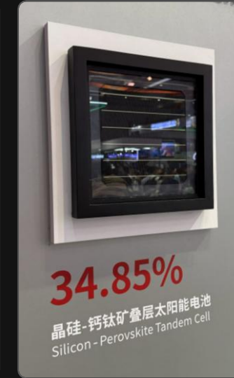
34.85% certified perovskite-silicon tandem cell (LONGi)
