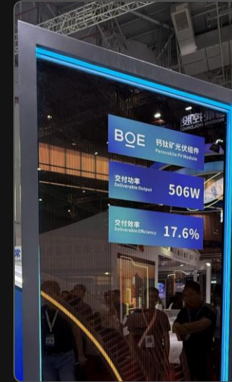
Full-size perovskite module: 506 W, 17.6% (BOE)
