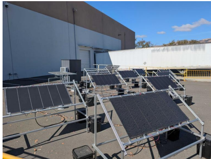
T20 pilot panels outdoors since July 2026; peak power stable (internal testing)
