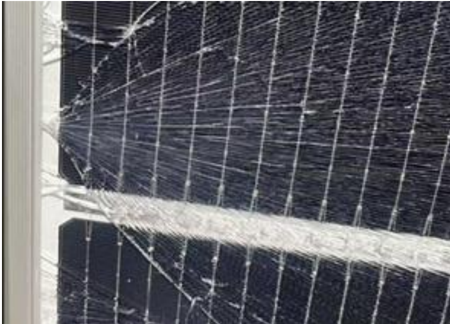
Module-1 broke during testing, showing a clear point of breakage due to edge pinch.
