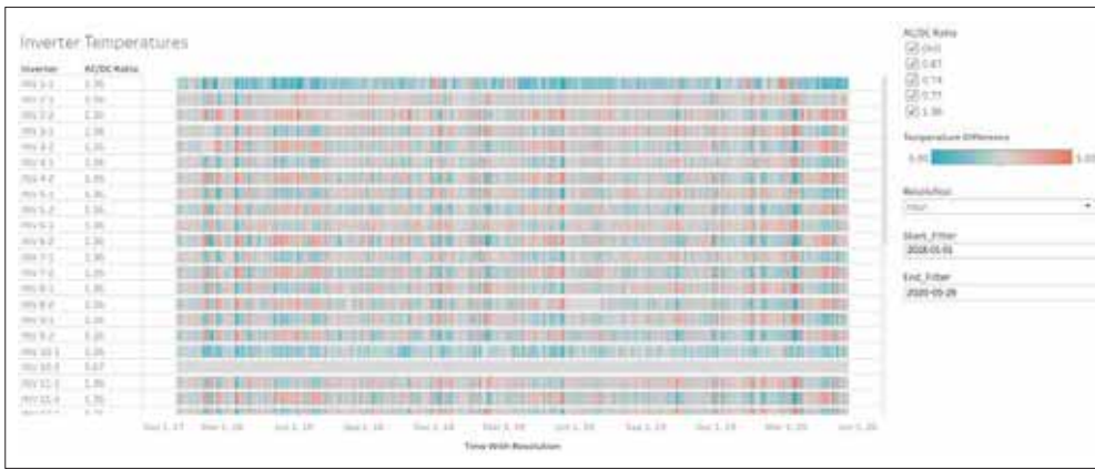
A chart showing the fluctuation of inverter temperatures on an operational solar system over time.
