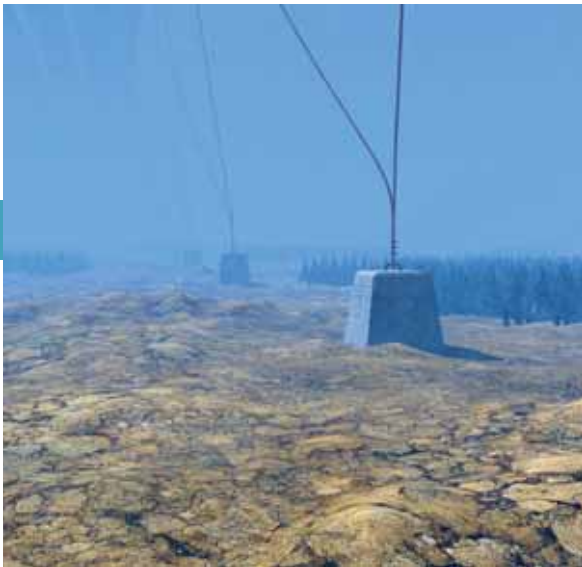
The design of special deadweight anchors used in the project.
